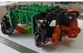
MARIA reactor weld joints UT scanning vehicle designed by Reactor and MRL engineers
