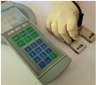
Magnetic Permeability Test according to IEC 60404-15 and ASTM
