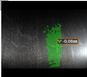
Cold drawing effects depth measurements Analysed by VT Flexible Videoendoscope
