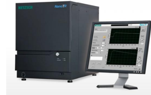
NanoTR enables measurements of thermal diffusivity of metallic, ceramic and composite layers in the range from 0.01 to 1000 mm 2 /s with an accuracy of 5%.
